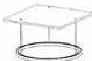
Step 06 Hang the circle by the steel wire
